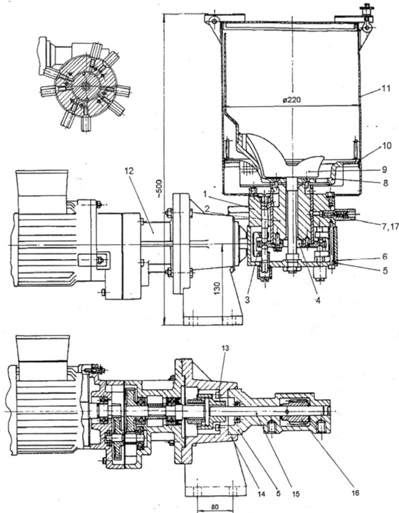
Fig. 2. Metering electro pump for consistent grease EPU 02.120.010.2
